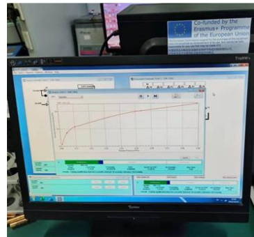
Micropore Automatic Physisorption Analyzer and computer for control, installed Room 207, Lab Building 17# of ECUST. Used to analyse the pore size distribution and the specific surface area of the materials, such as activated carbons.
